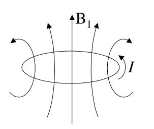
If unit current I produces a transverse RF field  $B_1$ , then transverse magnetization  $M_{xy}$  induces:
