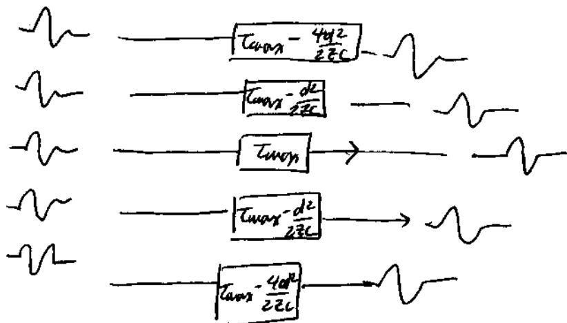
In practice, focusing achieved by a coarse time delay and a fine time delay / phase shift.
