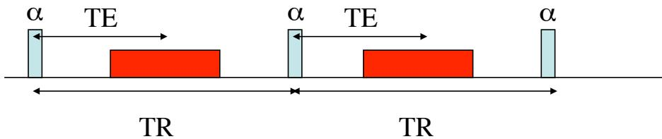
$$I(x,y) = \rho(x,y) \frac{\left[1 - e^{-TR/T_1(x,y)}\right] \sin \alpha}{\left[1 - e^{-TR/T_1(x,y)} \cos \alpha\right]} \exp(-TE/T_2^*)$$
